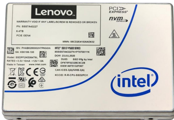
Figure 1. ThinkSystem Intel P5600 Mainstream NVMe PCIe 4.0 x4 SSD (shown without the ThinkSystem hot-swap tray)
