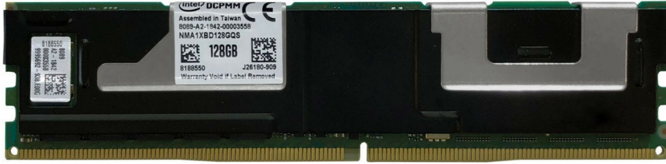
Figure 2. Intel Optane Persistent Memory
