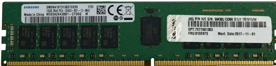
Figure 1. Lenovo TruDDR4 Memory DIMM
