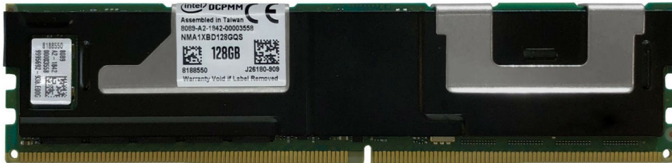
Figure 2. Intel Optane Persistent Memory
