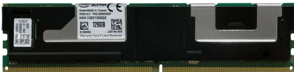
Figure 2. Intel Optane Persistent Memory
