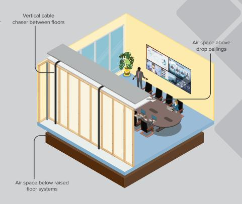
Low Smoke Zero Halogen cables are more easily disposed of, because they do not release harmful fumes into the environments as they do not contain any halogen elements (fluorine, chlorine, bromine, iodine and astatine).
