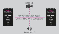
The HD-One DX series is available in HDBaseT and extended range variants in a compact form factor for the transmission of HDMI 1.4 signals including 1080p, 3D, UHD/4K and 4K DCI. Together, the HD-One DX series has full audio support including LPCM 7.1CH, Dolby, TrueHD, Dolby Digital Pluys and DTS-HD.
