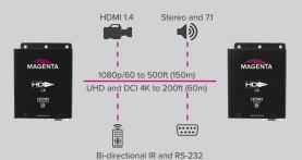
The HD-One LX series offers the same superior performance of the DX Series with additional support for bi-directional RS-232 and two-way, triple band infrared signals.
