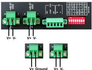
WARNING: The positive lead of the power source must be connected to the "+" terminal on the module and the negative lead of the power source to the "-" terminal on the module as shown above.
