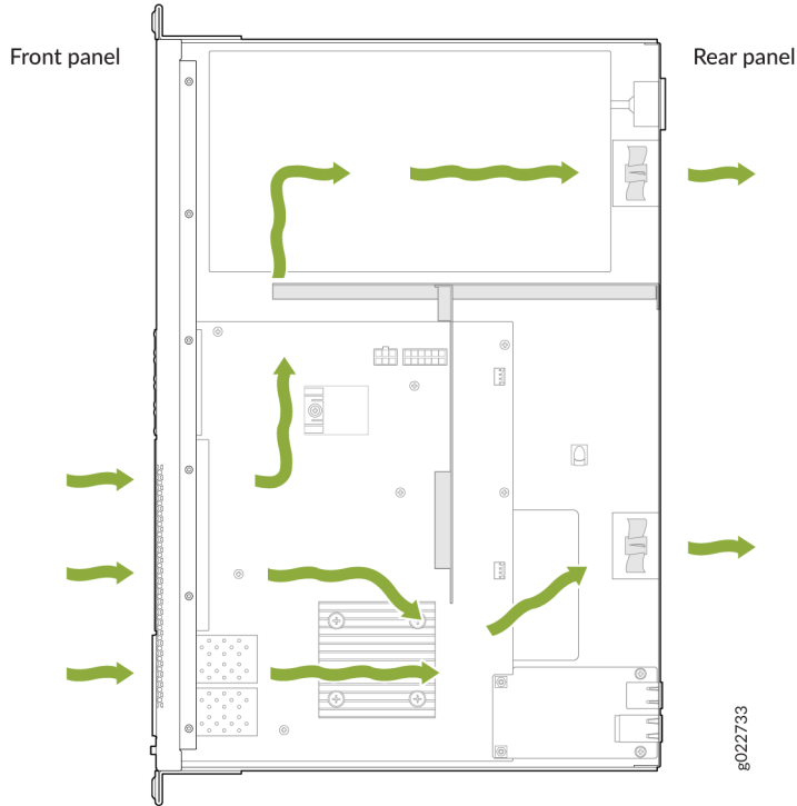
Figure 59: Front-to-Back Airflow Through the EX4100-F-24P Switch Chassis
