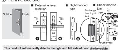
(how to set : It automatically sets when putting batteries. The door should be in open position.)
