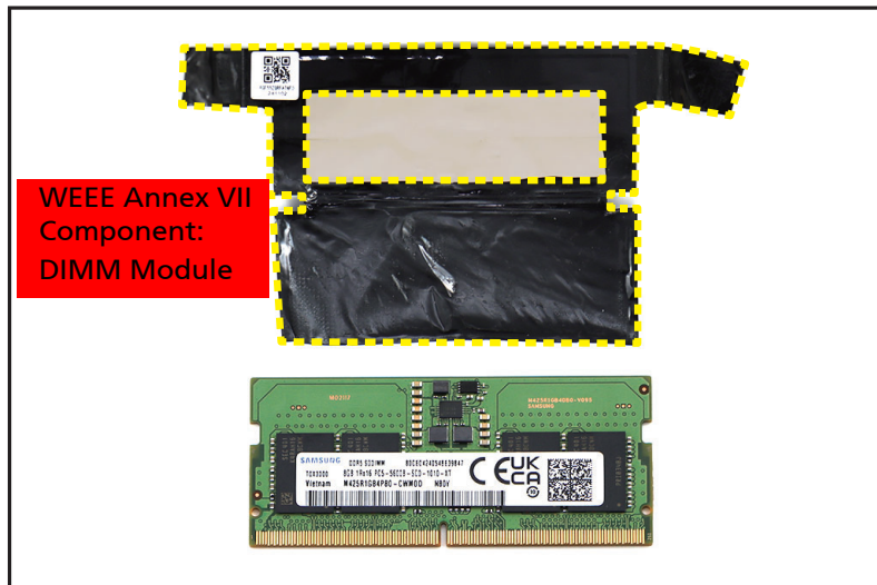
Figure 1-34. DIMM Module Removal
