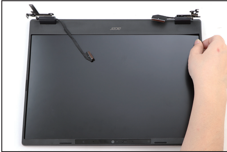
Figure 1-61. LCD Bezel Removal
