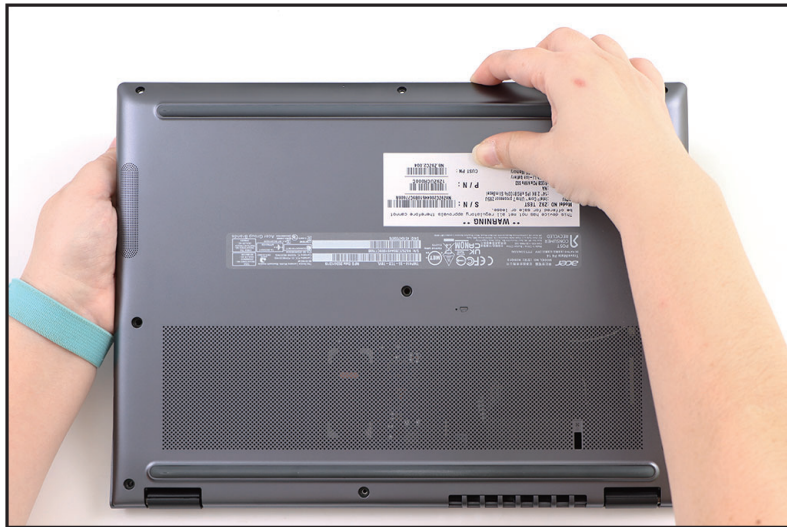
Figure 1-6. Base Cover Removal
