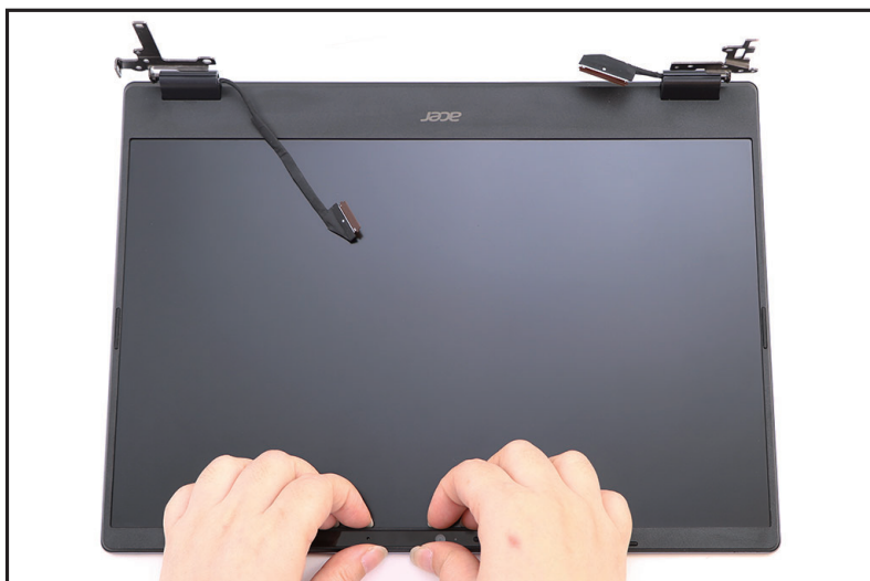
Figure 1-59. LCD Bezel Removal
