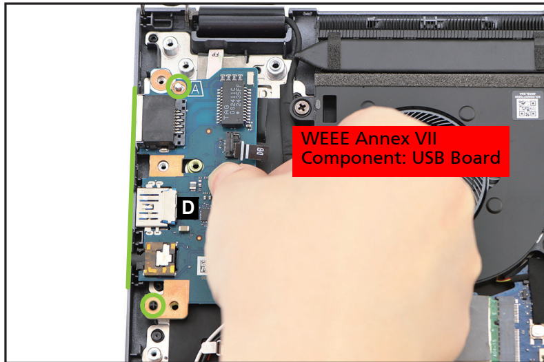
Figure 1-28. USB Board Removal
