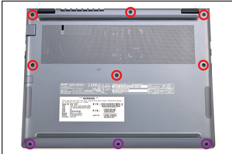
Figure 1-4. Base Cover Removal
