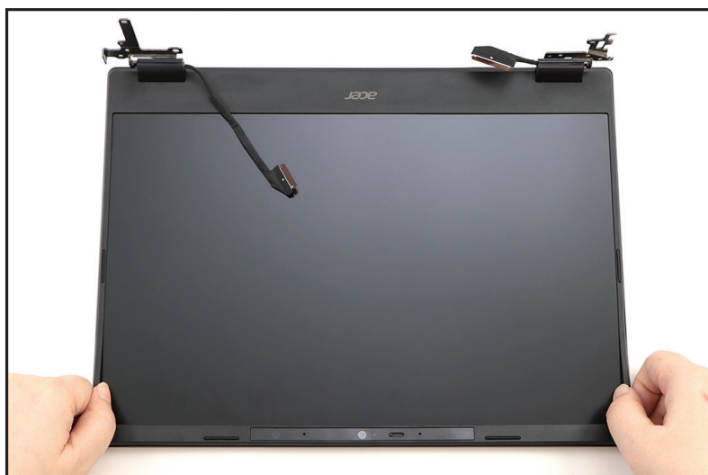
Figure 1-60. LCD Bezel Removal
