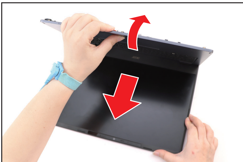
Figure 1-40. LCD Module Removal
