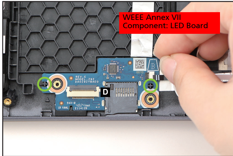
Figure 1-15. LED Board Removal
