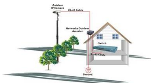
Fig. Addition an arrester between outdoor device and this switch
