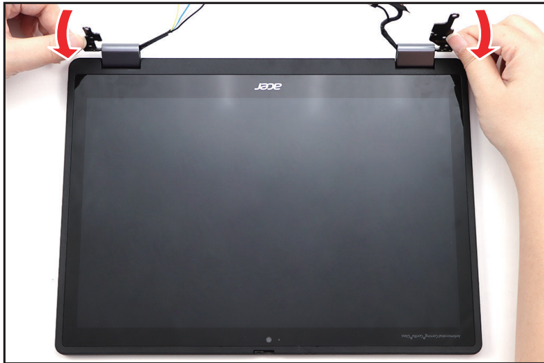
Figure 1-37. LCD Panel Removal
