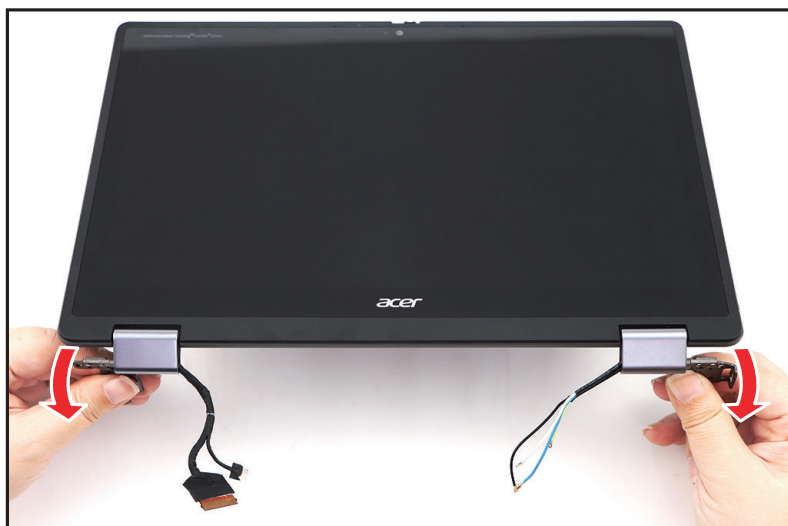
Figure 1-35. LCD Panel Removal
