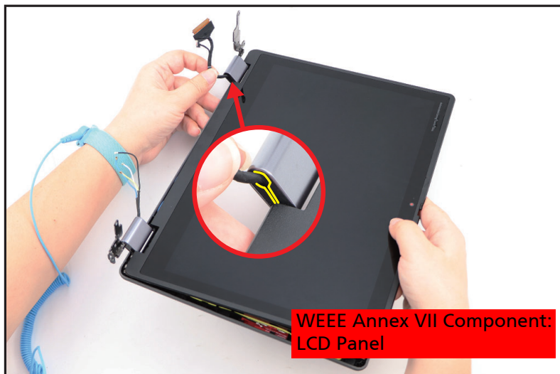
Figure 1-38. LCD Panel Removal
