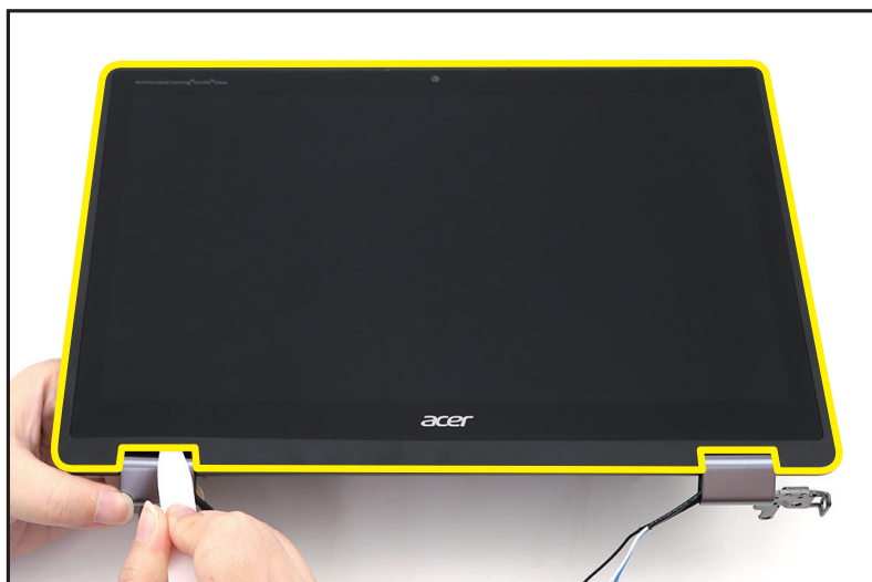
Figure 1-36. LCD Panel Removal
