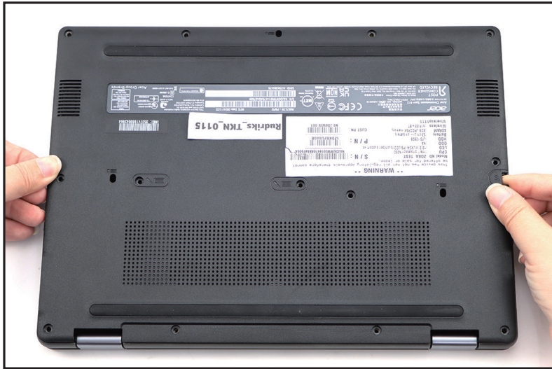
Figure 1-5. Base Cover Removal
