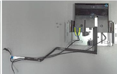
Rise up webcam, then remove webcam top cover
