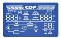
Shows input and output voltages, backup time and battery charge.
