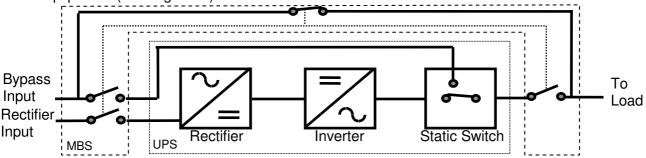
Figure 4. MBS in "Bypass" position
