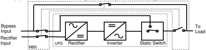
Figure 3. MBS in "Test" Position
