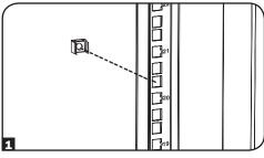
2 From the inside of the mounting rail, insert one of the flanges of the cage nut through the square opening. Press it against the side of the square opening. Each flange should engage one side of the square opening, not the top or bottom.
