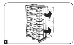
Remove the corner protectors. Save all packing materials (including the pallet) for later use unless you are certain they will not be required. The packing materials are recyclable.
