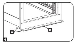
Use a 13 mm open-end wrench to remove the bolts attaching the enclosure to the shipping pallet. Be extremely careful, as the enclosure could shift unexpectedly after bolt removal. Save the reinforcing brackets and bracket hardware for later use.
