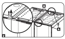
3 Loosen the bolt in each baying bracket and turn each bracket 180 degrees toward the adjoining enclosure, aligning each bracket with the corresponding baying connection point on the adjoining enclosure.
