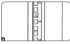
3 Compress the cage nut at the sides slightly to allow the remaining flange to fit through the square opening. When the cage nut is properly installed, both flanges will protrude through the square opening and will be visible on the outer surface of the mounting rail. Repeat steps 1-3 until all required cage nuts are installed.
