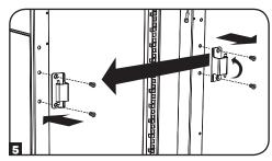
Unscrew the 2 hinge mechanisms from the hinge openings inside the door, then reattach each of them using the set of screw holes immediately opposite their original position.
