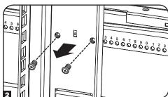
3 Slide the mounting rails to the desired depth and reattach them using the screws you removed in Step 2. The rail attachment points are numbered to help you align each pair of rails at the same depth.
