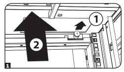
2 Remove the roof panel tabs **A** from the roof panel attachment slots **B** in the enclosure frame.
