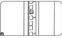
4 After installing the required cage nuts, use the included mounting screws and cup washers to secure your equipment to the rack rail. Place the cup washers between the screws and the equipment mounting brackets. Note: Your equipment may also include mounting hardware. Read the mounting instructions that came with your equipment before installing your equipment.
