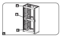
Remove the screws fastening each of the rear mounting rails to the enclosure. (If adjustment of the front rails is required, you can also remove the screws from the front rails.)
