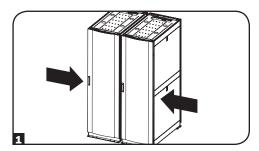
Each enclosure includes 2 baying brackets **A** that correspond to baying connection points **B** on the adjoining enclosure. The baying connection points already contain bolts. Remove the bolt and washer from each baying connection point in the adjoining enclosure.
