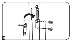
Rotate the door 180 degrees and reinstall it on the enclosure. Remember to connect the ground wire to the inside of the door, using the attachment point nearest the hinge at the top of the door. The attachment point is marked with the ground connection symbol:
