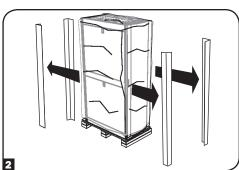
Remove the heavy plastic bag surrounding the enclosure. Examine the enclosure for any damage or loose parts. Confirm that all parts are present. If anything is missing or damaged, contact Tripp Lite for assistance. Do not attempt to use the enclosure if it has been damaged.
