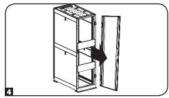
Remove the door hinges from the enclosure, rotate them 180 degrees and attach them on the opposite side of the enclosure. Note: The alternate door hinge attachment points have plastic plugs in the screw holes. Remove the plugs and insert them in the original door hinge attachment points.
