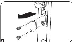
Remove the screw and washer from the rear of the door handle and remove the latching mechanism. Rotate the latch washer counter-clockwise 90 degrees and reverse the latch so it points in the opposite direction, then use the screw and washer to re-attach the latch to the rear of the door handle.
