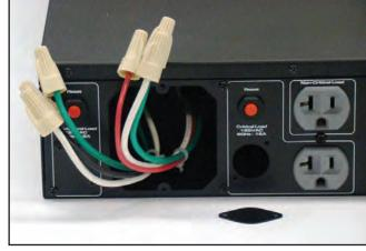
2) Insert cable connector (installer provided) while guiding conductors to the J-Box opening. Slide on lock-nut and and tighten on connector.
