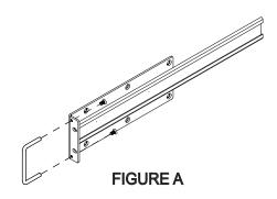
2) Install ears as shown using provided 10-32 screws. Six screws per ear, one ear per side.
