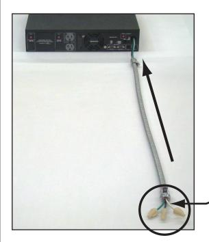
2) Grab and hold the three conductors at the end of the hardwired input cord (23). Gently slide the flexible conduit until the snap-in connector (24) meets the knock-out on the UPS.
