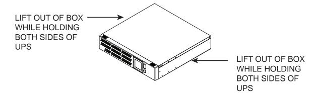
The UPS is very heavy and should be handled by two (2) people. After the product is removed from its shipping carton, inspect the UPS before installing and operating. The shipping carton should contain the following items:
