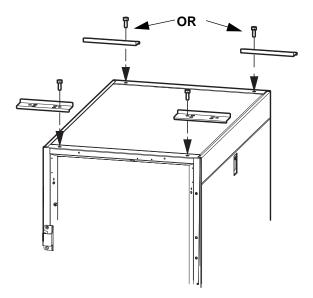
Roof brackets can be mounted on either side.
