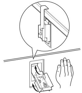
**9** Secure the two screws in the lock assembly.
