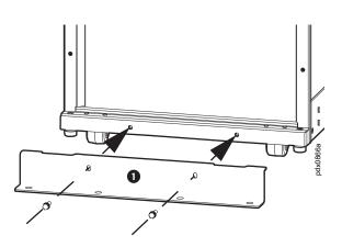
Secure the front anchoring bracket to the floor using floor anchoring bolts (not supplied). Use M12 strength class 8.8 or 1/2 inch, grade 5 steel bolts.
