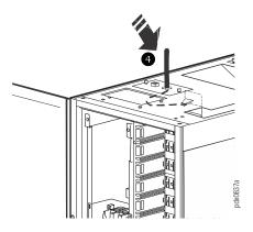
6 Make connections to the labelled terminals on the interface board.
