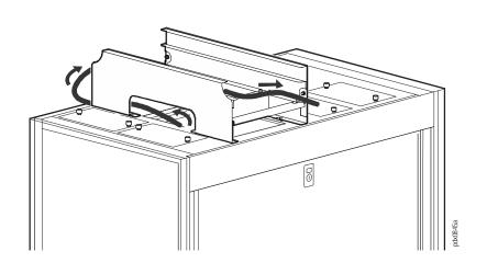
2 Feed PDM cables through the roof of the PDU and into the trough system for connection with the appropriate rack-mount PDUs.
