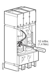
• Route the wires through the circuit breaker.
