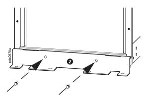
Push the PDU to slide the tabs on the bracket mounted to the PDU under the bracket bolted to the floor.
