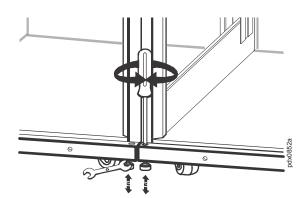
On not move the enclosure after the leveling feet have been lowered.
