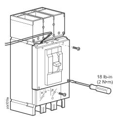
Remove the top plate and punch or drill an access hole for the Shunt Trip cable. Route the Shunt Trip cable through the top plate using appropriate strain relief.
