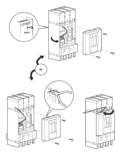
8 Replace the circuit breaker access cover. Torque the three screws to 18 lb-in (2 N•m).
