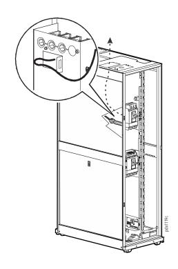
• Use the tie down slots on the inside of the PDU to attach cable ties and secure the Shunt Trip cable. Maintain proper spacing from power cables.
