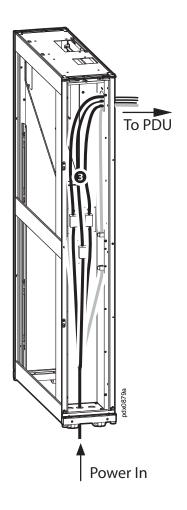
Connect the input/bypass conductors to the L1, L2, L3, EGC, and GEC terminals and torque to the specifications on the label.
