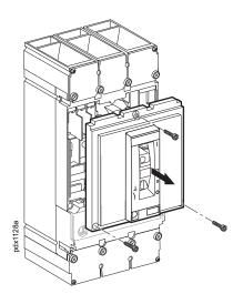
**9** Press the Shunt Trip into the lower left compartment of the circuit breaker, according to the manufacturer's instructions.
