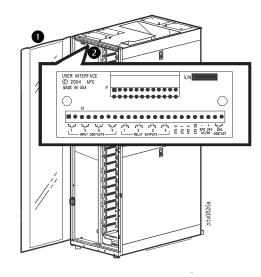
3 Loosen the captive screws and remove the plate. Remove the 3/4 in (19mm) knockout.
