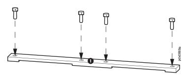
2 Secure the other half of the bracket assembly to the back of the unit.
