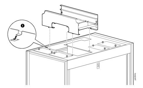
• Snap a Schneider Electric trough into slots on the roof of the PDU. The tabs at the base of the trough must fit securely into the slots.
