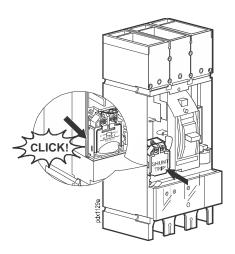
**⊙** Use the screwdriver to attach the wires to the Shunt Trip. Tighten the screws. Torque to 12 lb-in (1.4 N•m).
