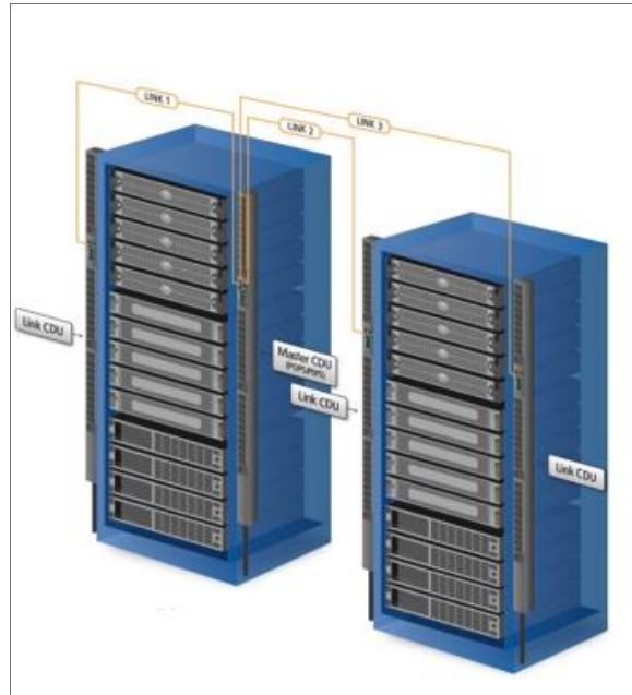
Multi-Linking View in the Equipment Cabinet
