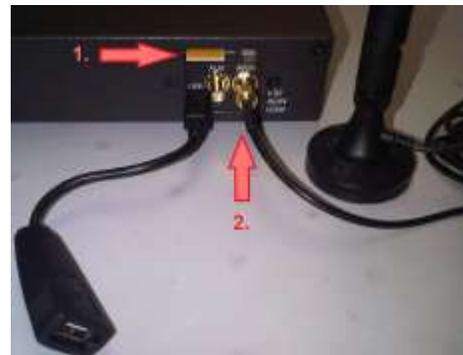
The IM4200-2-DAC-X2/X0-GV/GS and IM4216-34-DAC-X2-GV/GS models also have an internal cellular modem (and an internal 16GB flash memory and an additional USB port at the rear). They do not require a SIM card, but the supplied external antenna is installed as above. These models work with Verizon USA and Sprint USA respectively.
