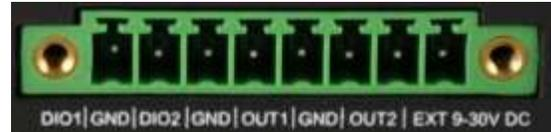
ACM7000 models ship with an in-built, black, spring cage I/O connector block for attaching environmental sensors and digital I/O devices.
