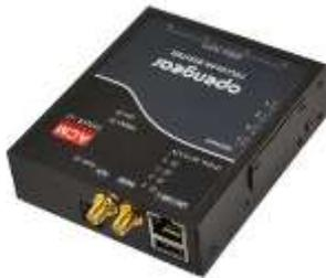
These models come with dual SMA antenna connectors. The AUX connector can be used for receive diversity. This requires an external antenna (accessory Part# 569006) and cable (Part# 449041).
