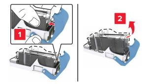
**4** Insert the new cartridge into the cartridge holder.
