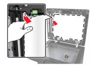
**3** Unpack the new ADF scan pad, and then remove the packing materials.
