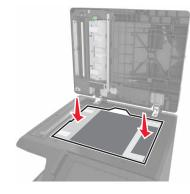
**5** Close the scanner cover to stick the ADF scan pad to the cover, and then open the cover.
