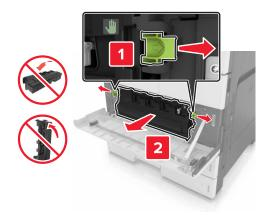
**3** Unlock the photoconductor unit.
