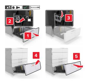
3 Open door C. Make sure that it does not hit any cable attached to the printer.Note: If the 3000-sheet tray is installed, slide the tray to open the door.
