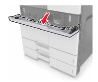
**2** Rotate the toner cartridge counterclockwise, and then pull it out.
