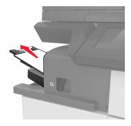
2 Press the latch on the staple finisher, and then slide the finisher to the left.
