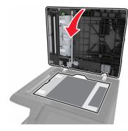
**6** Push the corners of the ADF scan pad to secure it into place.
