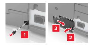
2 Remove the screws from the controller board access cover.
