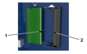
**4** Push the memory card straight into the connector, and then push the card toward the controller board wall until it *clicks* into place.
