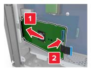
**c** Use the provided thumbscrew for the ISP to attach the ISP to the bracket.
