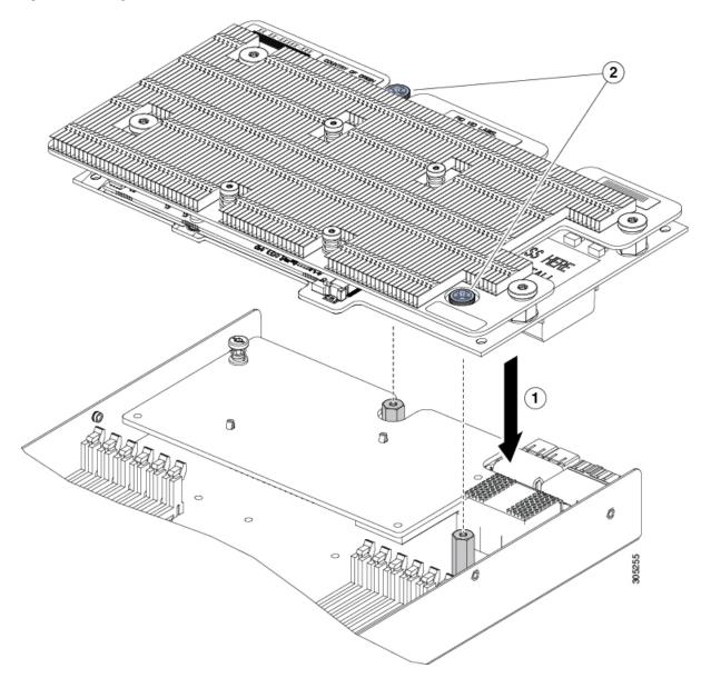
The following figure shows a GPU installed in a B200 M4 blade server.
