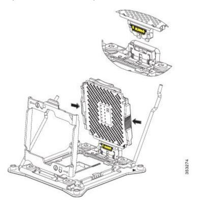
**Step 6** Pull the CPU carrier up and out of the SLS plug seat.
