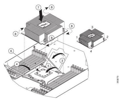
**Step 8** Tighten the four captive screws in the order shown.
