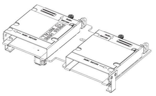
**Step 3** Using a Phillips-head screwdriver, tighten the four screws to secure the FlexStorage module. The locations of the screws are labeled "Secure Here."
