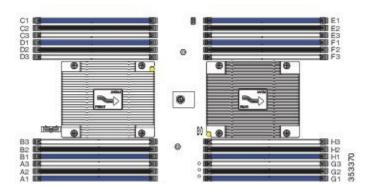
The figure below shows a logical view of the DIMMs and channels.
