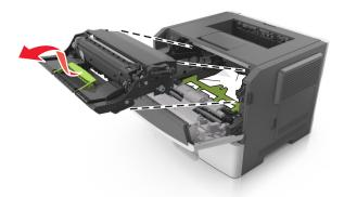
**Warning—Potential Damage:** Do not touch the shiny blue photoconductor drum under the imaging unit. Doing so may affect the quality of future print jobs.
