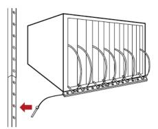
6. Repeat the above steps to connect additional blade extension strips and asset tags. Up to 128 asset tags on blade extension strips are supported per FEATURE port.
