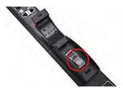
3. Push the cover of the fuse holder to expose the fuse.
