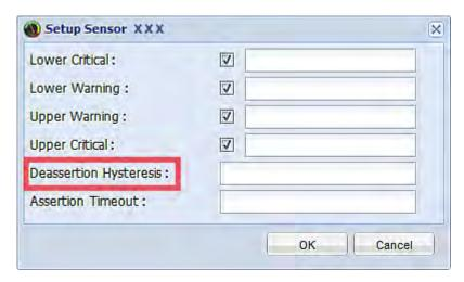
This function is similar to a thermostat, which instructs the air conditioner to turn on the cooling system when the temperature exceeds a pre-determined level. "Deassertion Hysteresis" instructs the PX to de-assert the worse state for a sensor only when that sensor's reading hits the pre-determined "deassertion" level.
