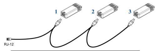
Tip: If the number of sensors you are connecting is less than the number of head connectors on your sensor cable, connect them to the first one or first two head connectors to ensure that there are NO free head connectors prior to the final DPX2 sensor attached.
