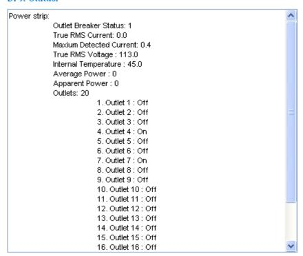
2. A status box appears, displaying details of the controlled PX, including power state of each outlet on the device.
