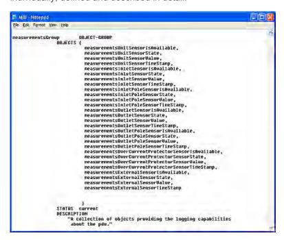
For example, the measurementsGroup group contains objects for sensor readings of PX as a whole. One object listed under this group, measurementsUnitSensorValue, is described later in the MIB as "The sensor value". pduRatedCurrent, part of the configGroup group, describes the PDU current rating.
