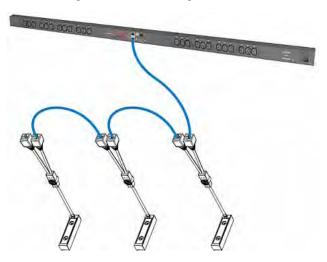
4. Repeat Step 2 to connect IT devices to the other composite asset sensors in the chain.
