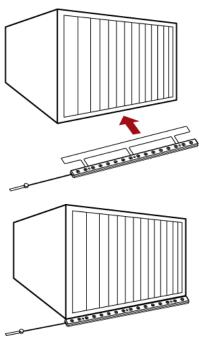
3. Connect one end of an asset tag to a blade server and connect the other end to the blade extension strip.
