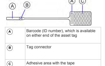
Note: The barcode of each asset tag is unique and is displayed in the PX device's web interface so it can easily be identified.
