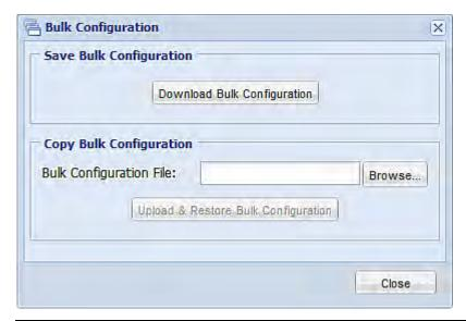
Note: No device-specific data is saved to the Bulk Configuration file, such as environmental sensor or certain network settings. To back up or restore a specific PX device's all settings, use the Backup/Restore feature instead. See Backup and Restore of PX Device Settings (on page 273).
