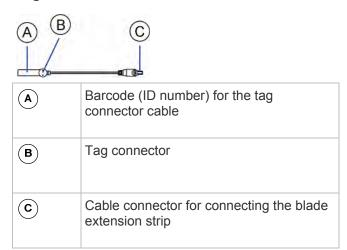
Note: A tag connector cable has a unique barcode, which is displayed in the PX device's web interface for identifying each blade extension strip where it is connected.
