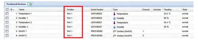
For DPX sensor series, the PX only displays the sensor port where it is physically connected.
