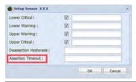
Note: For most sensors, the measurement unit in the "Assertion Timeout" field is sample. Because the PX measures each sensor every second, timing of a sample is equal to a second.
