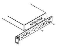
2. Insert the cable-support bar into rackmount brackets.
