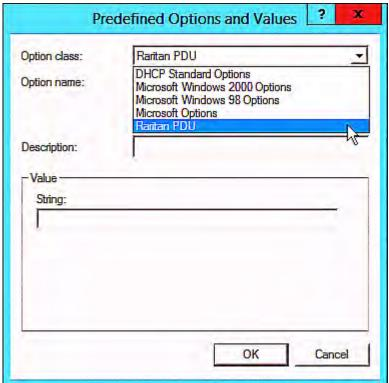
Click Add to add the first option. Type "pdu-tftp-server" in the Name field, select IP Address as the data type, and type 1 in the Code field.
