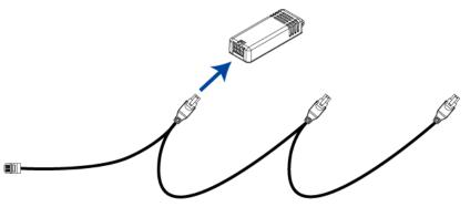
2. Connect remaining DPX2 sensors to the second and then the third head connector.
