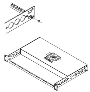
4. Fasten the rackmount brackets' ears to the rack using your own fasteners.
