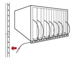
Repeat the above steps to connect additional blade extension strips. Up to 128 asset tags on blade extension strips are supported per FEATURE port.
