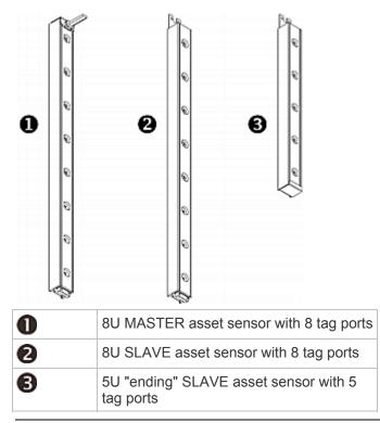
Note: Unlike general slave asset sensors, which have one DIN connector respectively on either end, the ending slave asset sensor has one DIN connector on only one end. An ending asset sensor is installed at the end of the asset sensor assembly.
