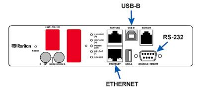
To use the command line interface (CLI) for configuration, establish an RS-232 or USB connection.
