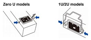
3. Connect the power cord to the inlet, and press the clip toward the power cord until it holds the cord firmly.
