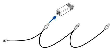
2. Connect remaining DPX2 sensor packages to the second and then the third head connector.
