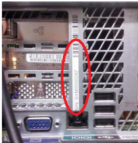
Figure 2-1 NetBackup 5230 Appliance serial number location
