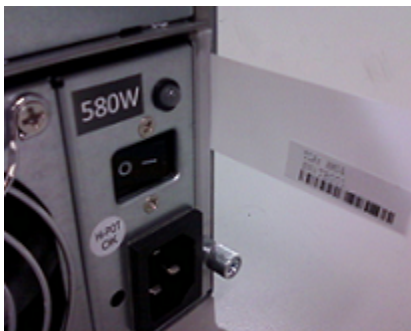
Figure 2-2 3U16 Storage Shelf serial number location
