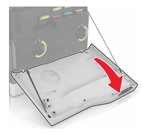
**3** Remove the keyboard attach cover.
