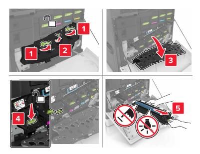
**4** Remove the photoconductor unit.
