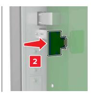
**Note:** The entire length of the connector on the card must touch and be flush against the controller board.
