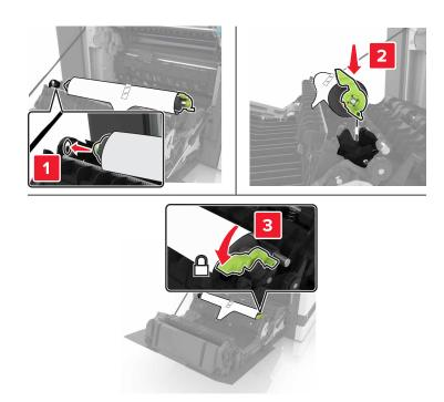
**5** Remove the white packing material.
