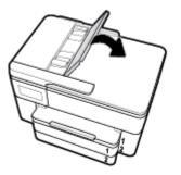
7. Lift the scanner lid to check, if there is jammed paper, remove it.
