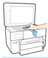
**CAUTION:** Use only glass cleaner to clean the scanner glass. Avoid cleaners that contain abrasives, acetone, benzene, and carbon tetrachloride, all of which can damage the scanner glass. Avoid isopropyl alcohol because it can leave streaks on the scanner glass.
