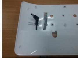
Route power and network cable from bottom, insert to signboard before mount signboard on back cover
