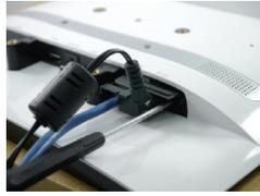
Fasten bracket onto the socket
