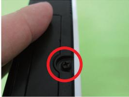
Release the back cover screw to release back cover
