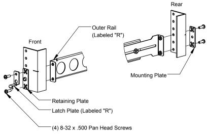
Step 4 <u>Install the Equipment:</u> Slide the equipment all the way in. Tighten the (2) Pan Head Screws on the back of the left slide rail. Slide the equipment out about 8 inches and tighten the (2) Pan Head Screws on the front of the left slide rail.
