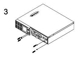
Remove the four retaining screws.
