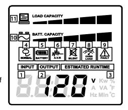
The LCD displays detailed information on the UPS status and current power conditions to alert you to potential power problems before the affect your equipment. Note! All related UPS information is based on that you should turn on the UPS.
