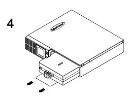
Insert the new battery pack. Assemble the screws, cable and front panel in the reverse sequence of above steps.\* Recharge the unit for 18 hours to ensure the UPS performs expected runtime.
