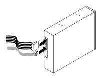
Figure 17. Connecting cables to the optical drive
