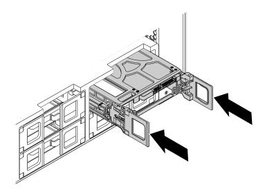
Figure 55. Installing the type 1 storage drive bracket
