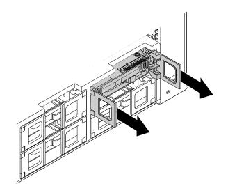
Figure 61. Removing the type **1** storage drive bracket
