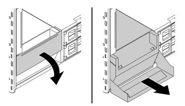
Figure 76. Removing the power supply assembly
