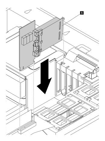
Figure 102. Installing the flex adapter
