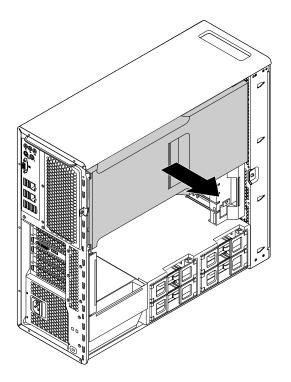
Figure 13. Removing the direct cooling air baffle
