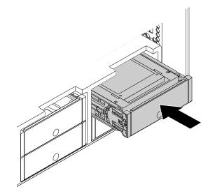
Figure 73. Installing the type 2 storage drive bracket
