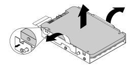
Figure 64. Removing the storage drive from the metal bracket of the converter
