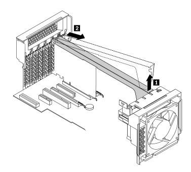
Figure 81. Removing the PCI card retainer
