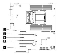
Figure 78. PCI Express card installation order for ThinkStation P510
