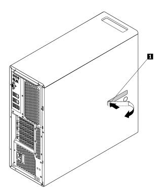
Figure 12. Removing the computer cover
