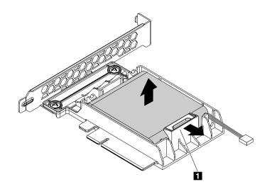
Figure 88. Removing the super capacitor module from the bracket
