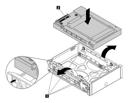
Figure 72. Installing the converter into the type 2 bracket
