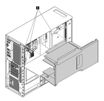
Figure 14. Installing the direct cooling air baffle
