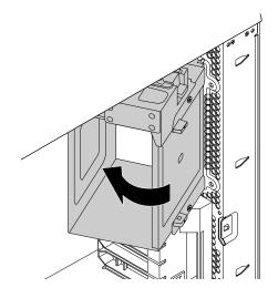
Figure 37. Installing the optical-drive bracket
