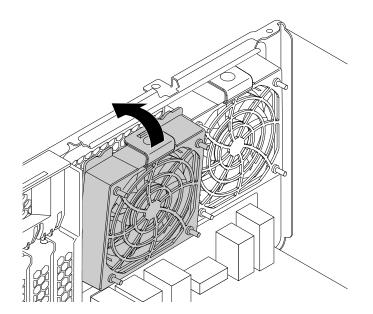
Figure 93. Installing the rear fan assembly
