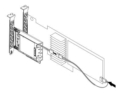
Figure 90. Connecting the super capacitor module cable
