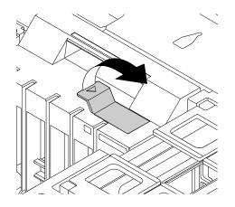
Figure 100. Opening the latch in the front fan assembly
