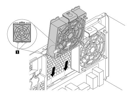
Figure 92. Positioning the rear fan assembly
