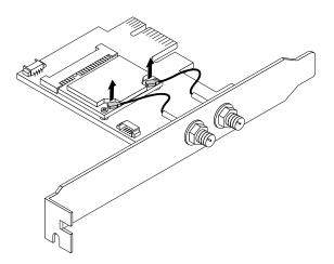
Figure 109. Disconnecting the Wi-Fi antenna cables
