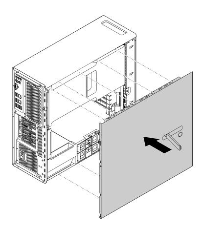
Figure 117. Positioning the computer cover
