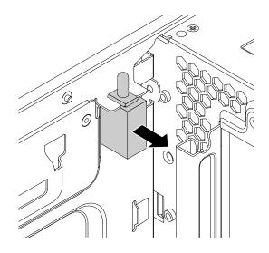
Figure 38. Removing the cover presence switch
