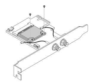
Figure 110. Removing the screws that secure the Wi-Fi card module
