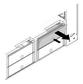
Figure 47. Removing the type 2 storage drive bracket
