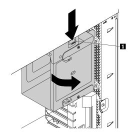
Figure 35. Removing the optical-drive bracket
