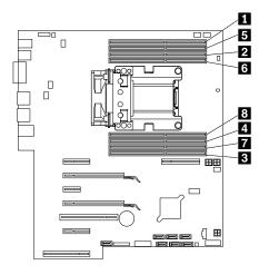
Figure 95. Memory module installation order for ThinkStation P510
