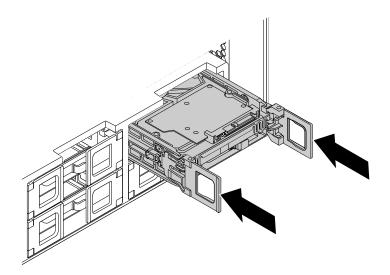
Figure 46. Installing the type 1 storage drive bracket
