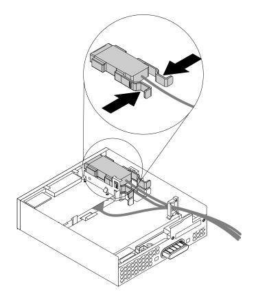
Figure 32. Removing the eSATA connector or IEEE 1394 connector in the flex module
