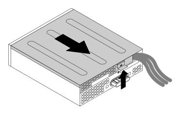
Figure 31. Removing the flex module cover
