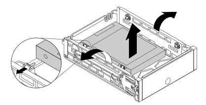
Figure 57. Removing the storage drive from the type 2 bracket
