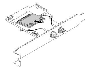
Figure 111. Removing the Wi-Fi card module
