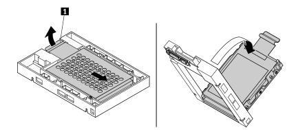
Figure 63. Removing the metal bracket from the plastic frame of the converter
