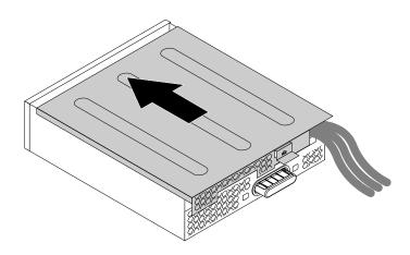
Figure 30. Reinstalling the flex module cover
