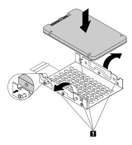
Figure 65. Installing the storage drive into the metal bracket of the converter
