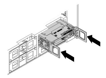
Figure 69. Installing the type 1 storage drive bracket
