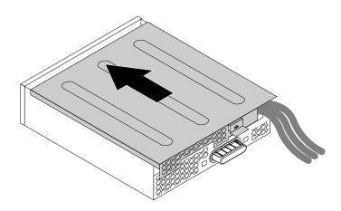
Figure 34. Reinstalling the flex module cover
