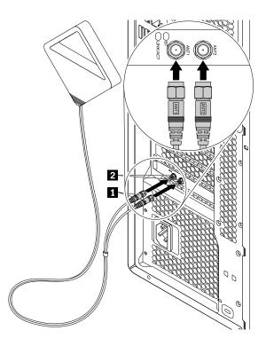
Figure 116. Installing the Wi-Fi antenna
