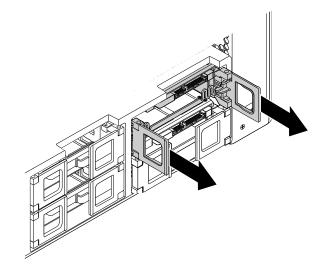
Figure 52. Removing the type 1 storage drive bracket
