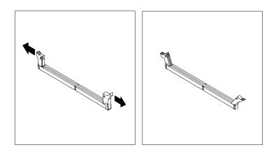
Figure 98. Opening the retaining clips
