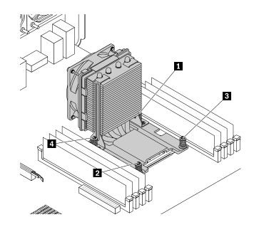
Figure 94. Removing the heat sink and fan assembly
