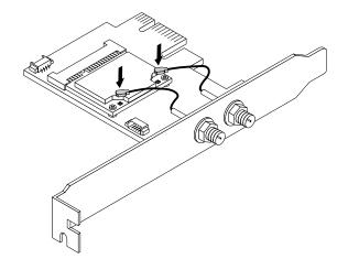
Figure 114. Connecting the Wi-Fi antenna cables
