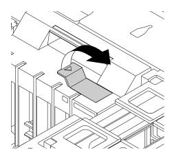
Figure 86. Opening the latch in the front fan assembly
