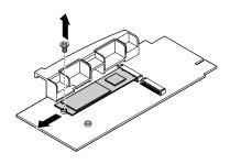
Figure 74. Removing the M.2 solid-state drive
