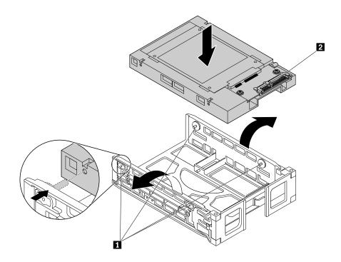
Figure 68. Installing the converter into the type 1 bracket
