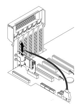
Figure 106. Disconnecting the Bluetooth cable
