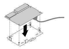
Figure 28. Installing the card reader into the card-reader retaining bracket
