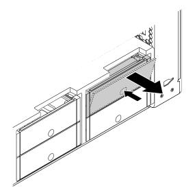
Figure 56. Removing the type 2 storage drive bracket
