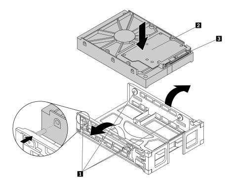
Figure 45. Installing the storage drive into the type 1 bracket
