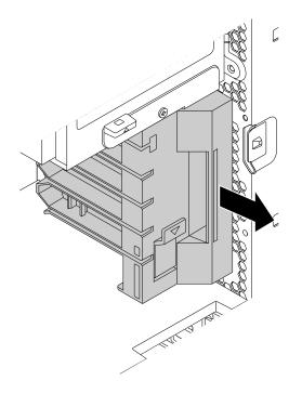
Figure 40. Removing the front fan assembly
