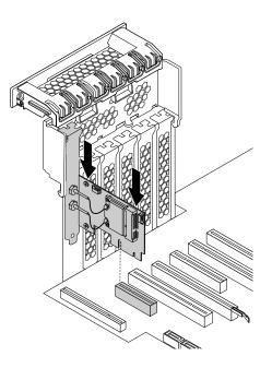
Figure 115. Installing the Wi-Fi adapter card
