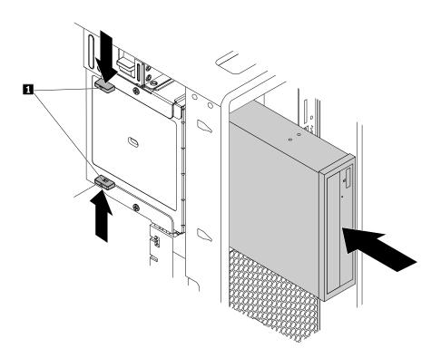
Figure 16. Installing the optical drive
