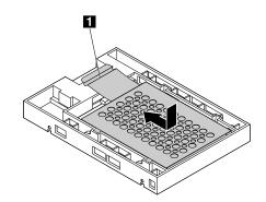
Figure 67. Installing the metal bracket into the plastic frame of the converter
