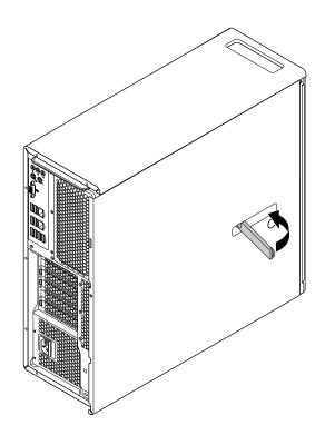
Figure 118. Reinstalling the computer cover
