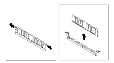
Figure 97. Removing a memory module
