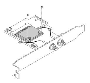
Figure 113. Installing the screws to secure the Wi-Fi card module
