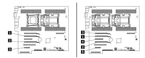
Figure 79. PCI Express card installation order for ThinkStation P710
