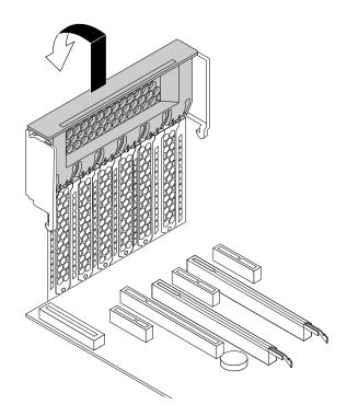
Figure 85. Opening the PCI card latch
