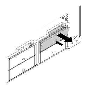
Figure 70. Removing the type 2 storage drive bracket
