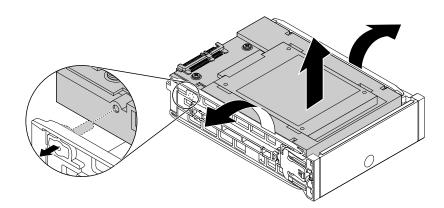
Figure 71. Removing the converter from the type 2 bracket
