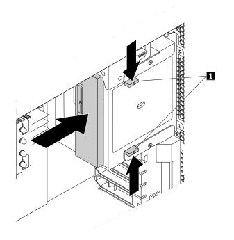
Figure 15. Removing the optical drive
