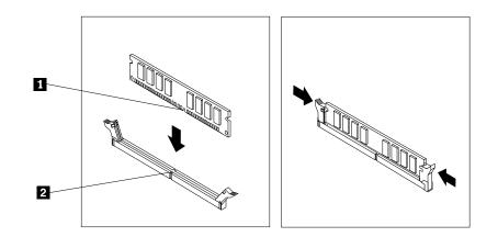
Figure 99. Installing a memory module
