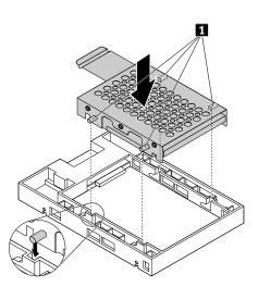
Figure 66. Inserting the metal bracket into the plastic frame of the converter
