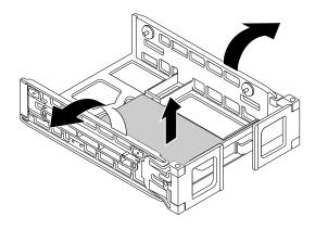
Figure 53. Removing the storage drive from the type 1 bracket
