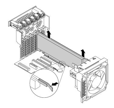
Figure 87. Removing a full-length PCI card
