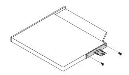
Figure 21. Removing the plastic clip from the slim optical drive
