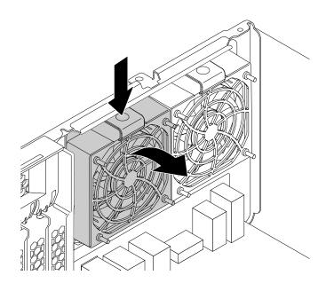
Figure 91. Removing the rear fan assembly
