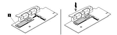
Figure 75. Installing the M.2 solid-state drive
