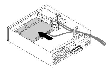
Figure 29. Installing the card reader in the flex module
