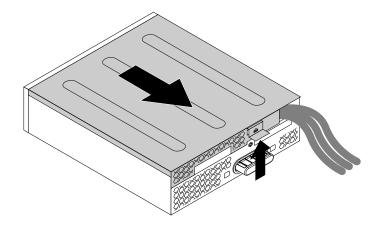
Figure 18. Removing the flex module cover
