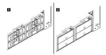
Figure 60. Two types of storage drive bracket
