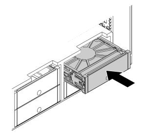
Figure 50. Installing the type 2 storage drive bracket
