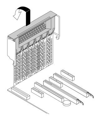
Figure 82. Opening the PCI card latch
