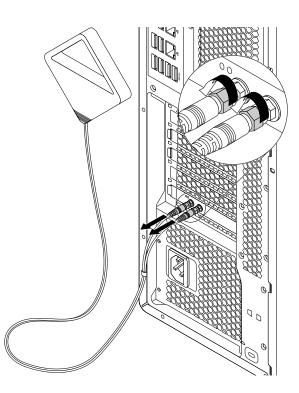
Figure 105. Removing the rear Wi-Fi antenna
