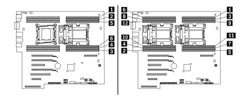
Figure 96. Memory module installation order for ThinkStation P710
