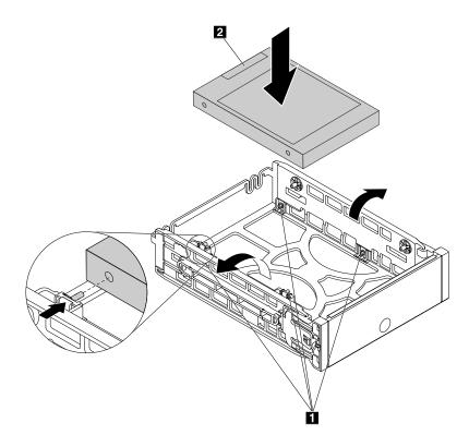
Figure 58. Installing the storage drive into the type 2 bracket
