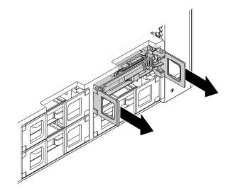
Figure 43. Removing the type 1 storage drive bracket
