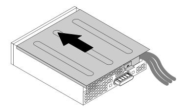
Figure 24. Reinstalling the flex module cover
