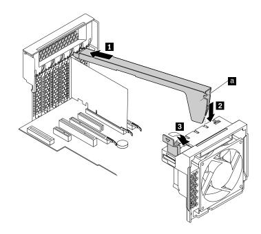
Figure 84. Installing the PCI card retainer
