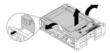
Figure 62. Removing the converter from the type 1 bracket
