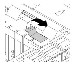
Figure 80. Opening the latch in the front fan assembly
