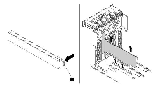
Figure 83. Removing a PCI card
