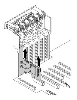
Figure 108. Removing the Wi-Fi adapter card
