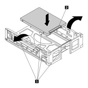
Figure 54. Installing the storage drive into the type 1 bracket
