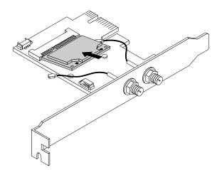
Figure 112. Installing the Wi-Fi card module
