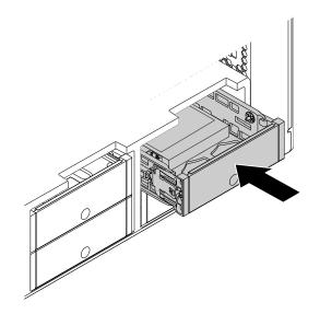
Figure 59. Installing the type 2 storage drive bracket
