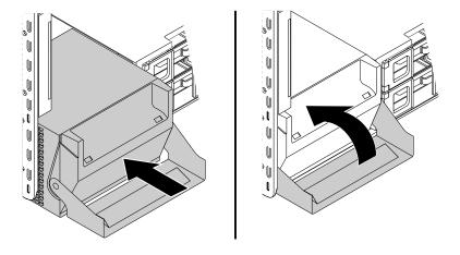
Figure 77. Installing the power supply assembly
