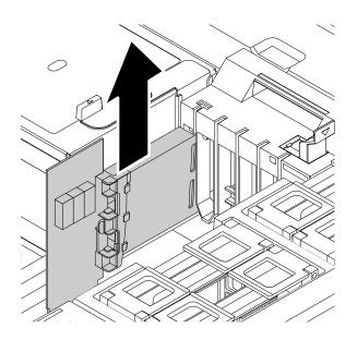
Figure 101. Removing the flex adapter
