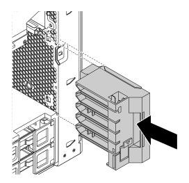
Figure 41. Installing the front fan assembly
