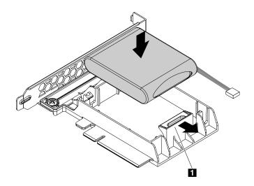
Figure 89. Installing the super capacitor module into the bracket
