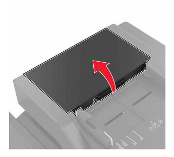
**3** Remove the ADF separator roller cover.
