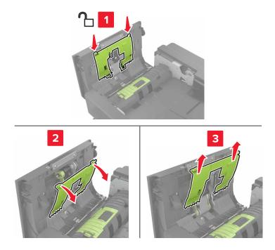
4 Remove the ADF feed roller.
