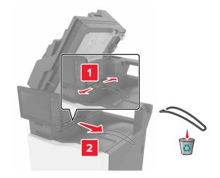
Remove the paper transport and staple finisher connector covers.
