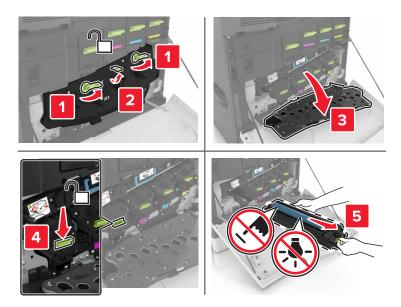
**5** Unpack the new imaging unit, and then remove the packing material.
