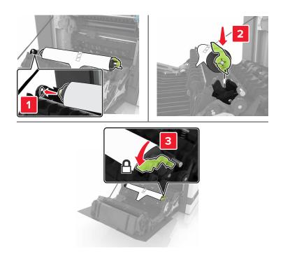
**5** Remove the white packing material.
