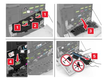
Remove the photoconductor unit.
