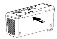
3 Connect the battery cable securely to the battery terminal. It is normal for small sparks to be seen when the battery cable is connected to the battery terminal.
