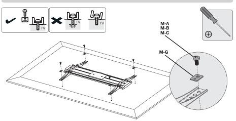
**Note:** Choose the appropriate Screws, Washers and Spacers (if needed) according to the type of screen. Screw the Adapter Brackets onto the display.
