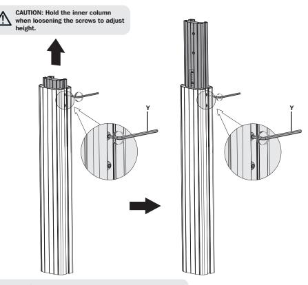
Adjust inner Column J to the desired height, then tighten all screws.
