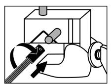
To use clamp aligned vertically, screw gooseneck onto the male metal connection bolt on the side of the clamp.
