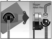
Use the bigger Allen key to tighten and loosen the gooseneck to holder connection, adjusting ease of rotation.
