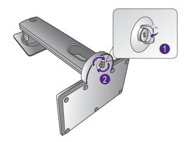
Orient and align the stand arm with the monitor (1), push them together until they click and lock into place (2).
