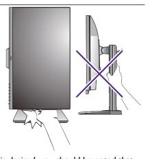
• If the monitor has been rotated to portrait mode and height adjustment is desired, you should be noted that the wide screen will keep the monitor from being lowered to its minimum height.
