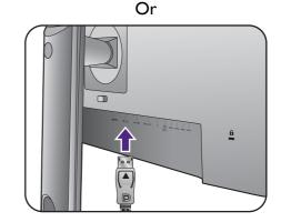
After the monitor and the computer are powered on, if the image is not displayed, disconnect the DP cable. Connect the monitor to any video source other than DP first. Go to **System** and **DisplayPort** on the OSD menu of the monitor and change the setting from **1.2** to **1.1**. Once the setting is done, unplug the current video cable and re-connect the DP cable. To go to the OSD menu, see Basic menu operation on page 28.
