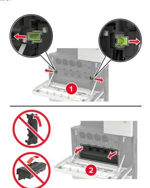
Using the printhead wiper, clean the printhead lens.
