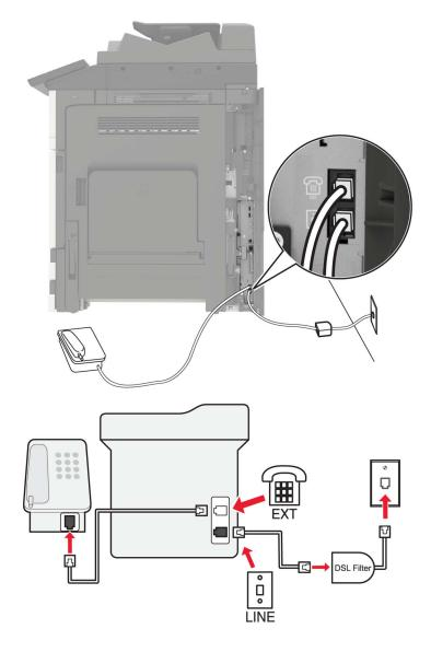
Digital subscriber line (DSL) splits your regular telephone line into two channels: voice and Internet. Telephone and fax signals travel through the voice channel, and Internet signals pass through the other channel.
