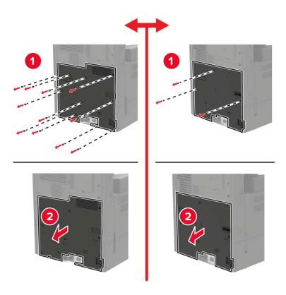
**5** Remove the controller board shield.
