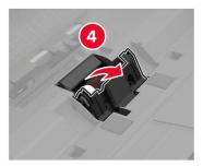
Remove the ADF separator roller.
