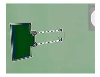
**Note:** The entire length of the connector on the card must touch and be flush against the controller board.
