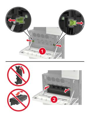
**3** Remove the photoconductor unit.
