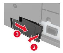
4 Remove the controller board access cover.
