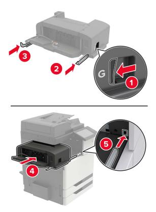
Secure the finisher to the printer.
