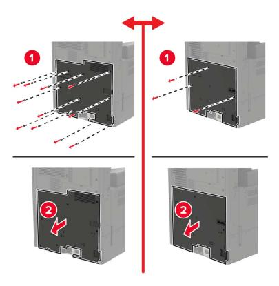
Remove the controller board shield.
