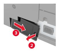
**4** Remove the controller board access cover.
