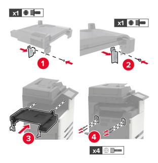
Attach the finisher to the printer.
