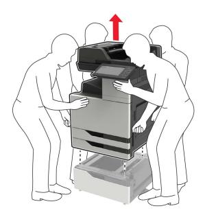
Remove the stabilizing feet from the tray.
