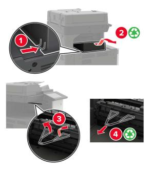
Using the screwdriver stored inside door A, remove the paper guides.
