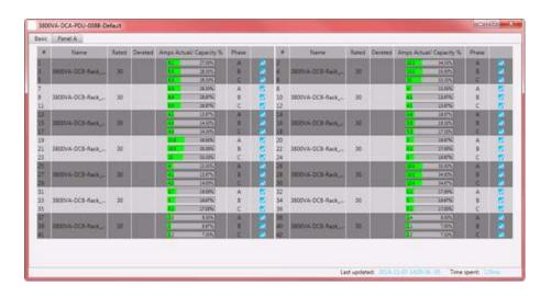
The PDU Smart Interface is a dashboard view that allows users to see a PDU with breakers broken up and composed of individual circuits. Based upon values entered by the user and live data being collected, ampere water capacity gauges self-populate showing a percentage utilized image to viewers.
