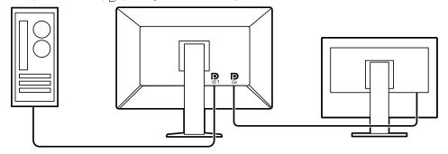
• In order to display images in PbyP, two signal cables usually need to be connected between the PC and the monitor. On this model, you can connect it to the PC using one cable. You only need to connect the supplied DisplayPort cable (PP028) between the output terminal ( ) and the input terminal ( ).
