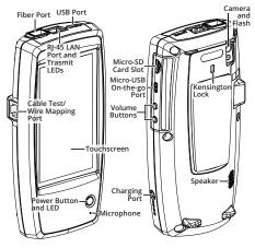
The LinkRunner G2 is an Android-based network testing and troubleshooting tool. It allows networking professionals to easily verify network connectivity and PoE functionality and to validate cabling. LinkRunner G2 can also act as a packet reflector for performance tests run by other netAlly testers and includes a VLAN Monitor and packet Capture tools.
