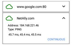
The expanded Target Test card shows the IP address of the target, the type of test (Ping or
