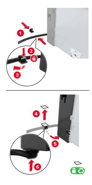
Connect the tray cable to the printer.
