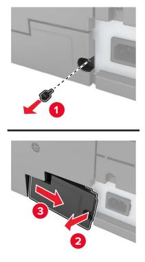
**4** Remove the controller board access cover.
