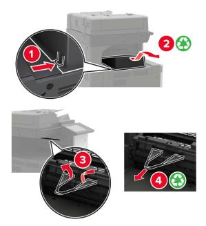
**6** Using the screwdriver stored inside door A, remove the paper guides.
