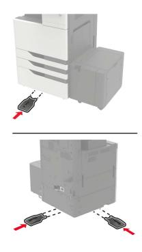
**22** Connect the 2 x 500- or 2500-sheet tray connector to the printer.
