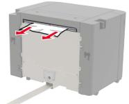
3 Open door F, and then remove the jammed paper.Note: Make sure that all paper fragments are removed.
