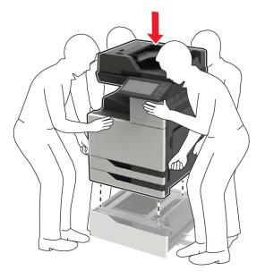
**16** Align the 3000-sheet tray with the printer, and then attach the mounting post.
