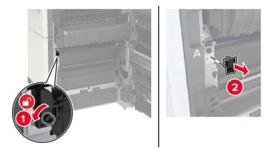
**4** Loosen the screws that secure the transfer belt.
