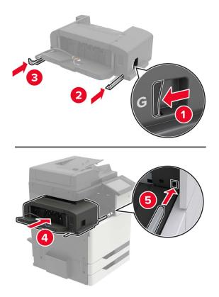
**10** Secure the finisher to the printer.
