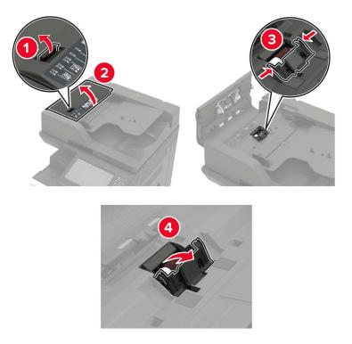
**3** Remove the ADF separator roller.
