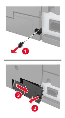
**4** Remove the controller board access cover.
