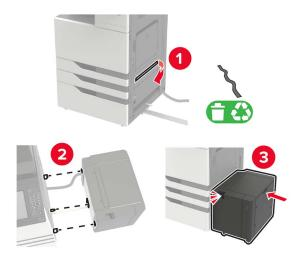
Attach the stabilizing feet to the printer.
