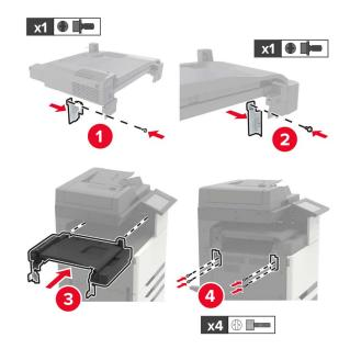
Attach the finisher to the printer.
