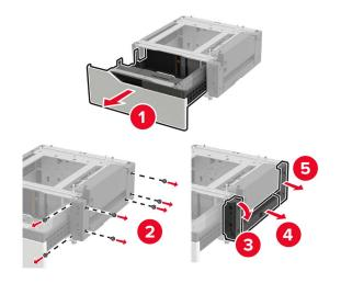
**12** Attach the side mounting brackets to the tray, and then insert the guide plate into the rail.
