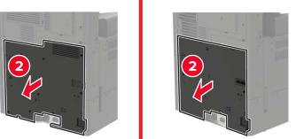
**5** Remove the controller board shield.
