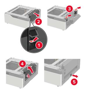
**11** Open the tray, and then remove the mounting bracket and rail covers.
