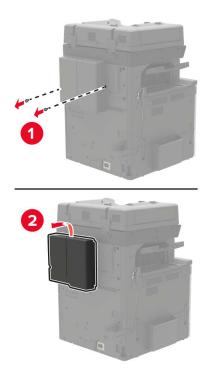
**11** Connect the finisher cable to the printer.
