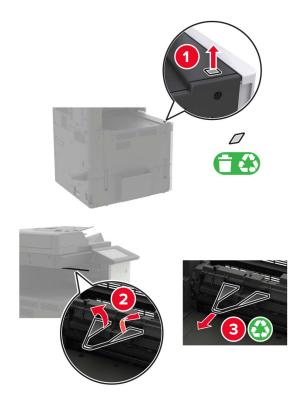
**6** Using the screwdriver stored inside door A, remove the covers for the paper guide sensor and slide rail.
