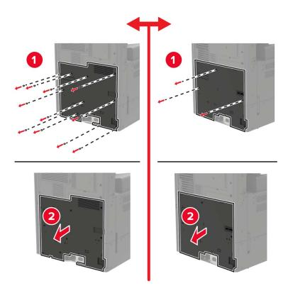
**5** Remove the controller board shield.
