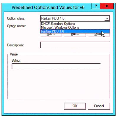
c. Click Add to add the first option. Type "pdu-tftp-server" in the Name field, select IP Address as the data type, and type 1 in the Code field.
