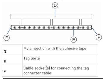
Note: Each tag port on the blade extension strip is labeled a number, which is displayed as the slot number in the PX2 device's web interface.
