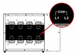
In all 3-phase products, L1 is phase A, L2 is phase B, L3 is phase C and N is neutral.
