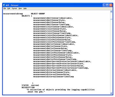
For example, the measurementsGroup group contains objects for sensor readings of PX2 as a whole. One object listed under this group, measurementsUnitSensorValue, is described later in the MIB as "The sensor value". pduRatedCurrent, part of the configGroup group, describes the PDU current rating.
