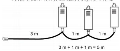
The total cabling length between the PX2 and one DPX-T3H1 is 49'
