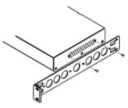
2. Insert the cable-support bar into rackmount brackets.
