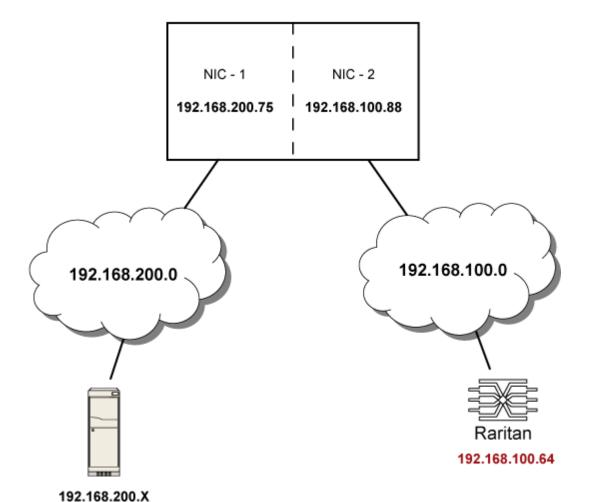
In this example, NIC-2 (192.168.100.88) is the next hop router for your PX2 to communicate with any device in the other subnet 192.168.200.0. In the IPv4 "Static Routes" section, you should enter the data as shown below. Note that the address in the first field must be of the Classless Inter-Domain Routing (CIDR) notation.
