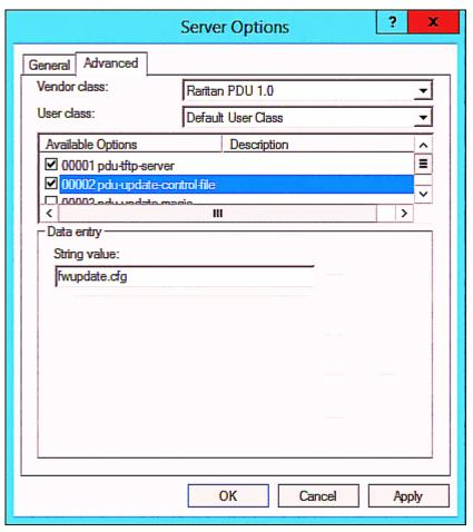
e. Select "00003 pdu-update-magic" from the Available Options list, and type any string in the "String value" field. This third option/code is the magic cookie to prevent the *fwupdate.cfg* commands from being executed repeatedly. It does NOT matter whether the IPv6 magic cookie is identical to or different from the IPv4 magic cookie.
