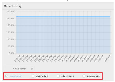
When multiple outlets are displayed in the chart, their data lines' colors differ. You can identify their lines according to the colors of the selected outlet checkboxes as illustrated below.
