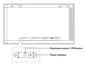
Illuminance sensor: Adjusts the screen brightness by measuring the amount of light.
