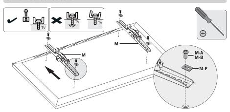
**Note:** Choose the appropriate Screws, Washers and Spacers (if needed) according to the type of screen. Screw the Mounting Arms onto the display.
