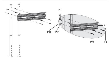
Insert Washers P-F and Nuts P-H into rear of Telescoping Poles H at desired height. Secure Universal Plate J with Screws P-C using Allen Wrench P-J.
