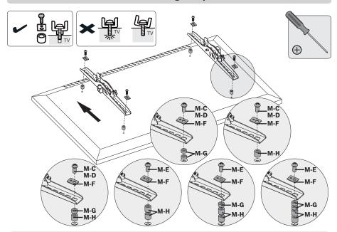
**Note:** Choose the appropriate Screws, Washers and Spacers (if needed) according to the type of screen. Screw the Mounting Arms onto the display.
