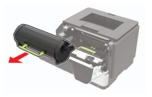
**3** Remove the used imaging unit.
