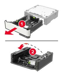
Remove the used pick roller assembly.
