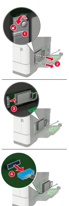
**b** Connect the ISP extended cable to the ISP connector.
