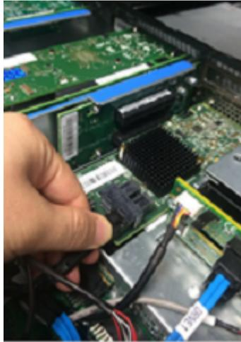
**15** Replace the air duct. Be sure that the small clear tabs on the air duct arms sit firmly under the blue lifting frames.
