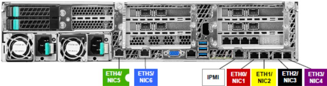
By default, NIC1 (eth0) is factory set to IP address 192.168.229.233. This private network address is reserved to provide a direct connection from a laptop to perform the initial configuration. NIC1 (eth0) is typically not connected to your network environment.
