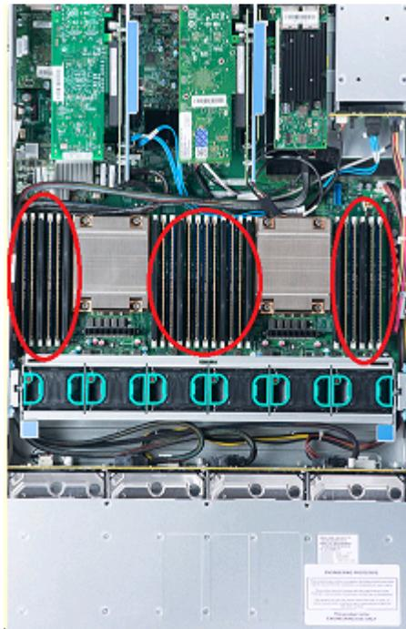
Each DIMM socket has an identifier on the main board that consists of a two-digit alphanumeric character that indicates the channel and socket for each DIMM. Socket identifiers have the format A1, A2, B1, B2, C1, C2, etc. The letter defines the channel and the number indicates the socket.
