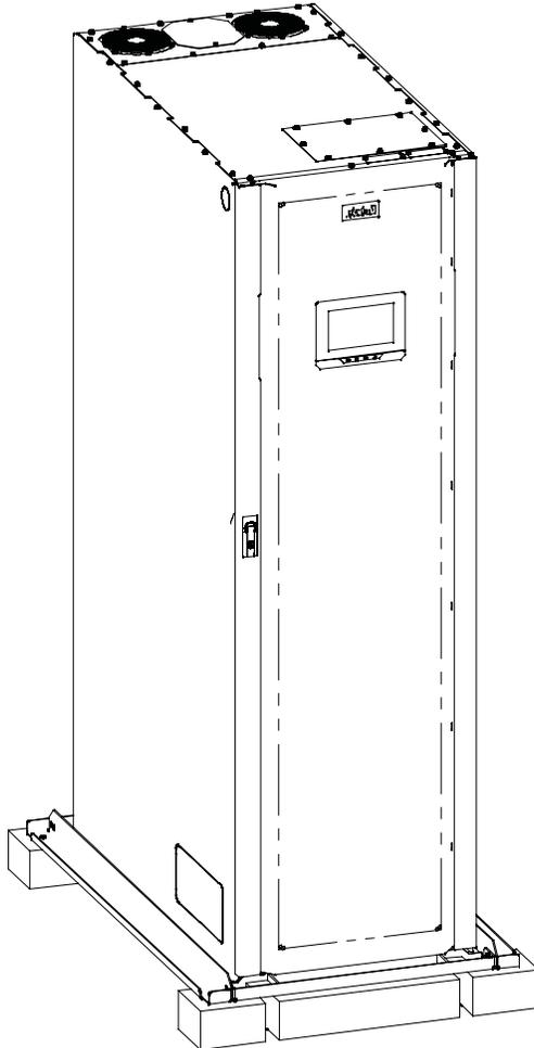
**Figure 3-10. UPS Cabinet as Shipped on Pallet**
